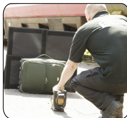
Large Format Flexi Plates for large area x-ray investigation
