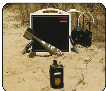
Rugged, weather- resistant flat panel aSi x-ray imagers.
